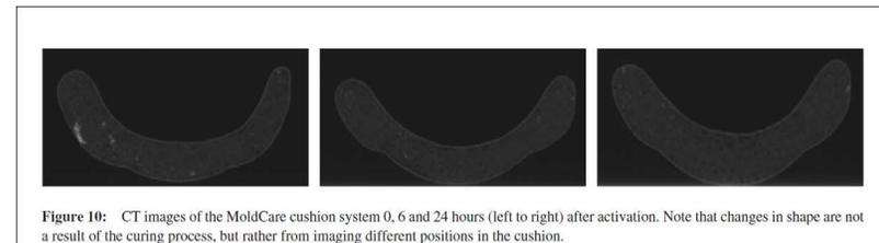
Figure 10: CT images of the MoldCare cushion system 0, 6 and 24 hours (left to right) after activation. Note that changes in shape are not a result of the curing process, but rather from imaging different positions in the cushion.
